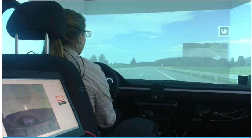
Car Driving Simulator with Eye-Tracking at OFFIS
